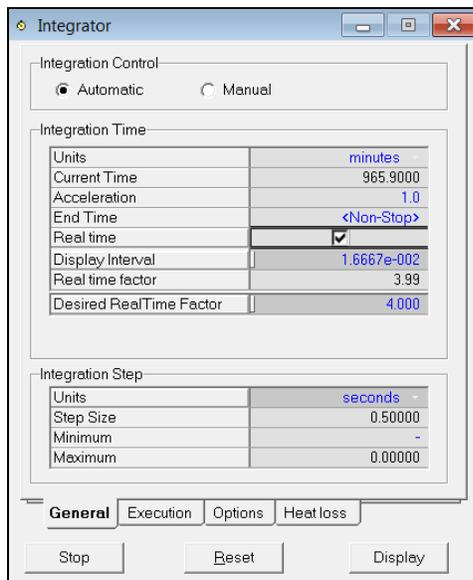
For the OTS, Inprocess normally uses a step size in the range of 0.1 to 0.5, but specific scenarios may require a different (typically lower) time step. You should also keep in mind to correctly specify the execution rates on the “Execution” page of the integrator.
