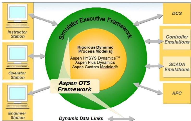
Figure 1: Aspen Simulation Executive Framework Diagram
