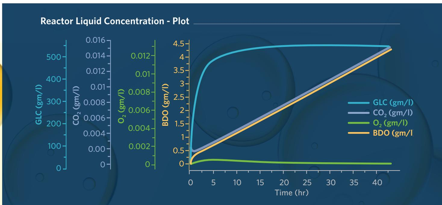
Figure 2. Aspen Plus generated composition plot shows the liquid phase concentration changes within the reactor through the reaction time. GLC here refers to the concentration of glucose as it builds up in the reactor.
