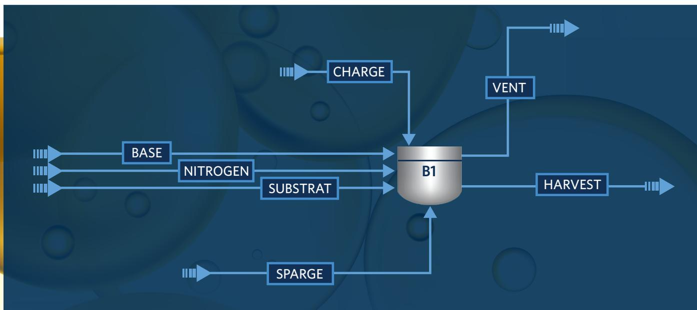
Figure 1. Semi-batch bioreactor inputs and outputs to produce 1,4-butanediol.
