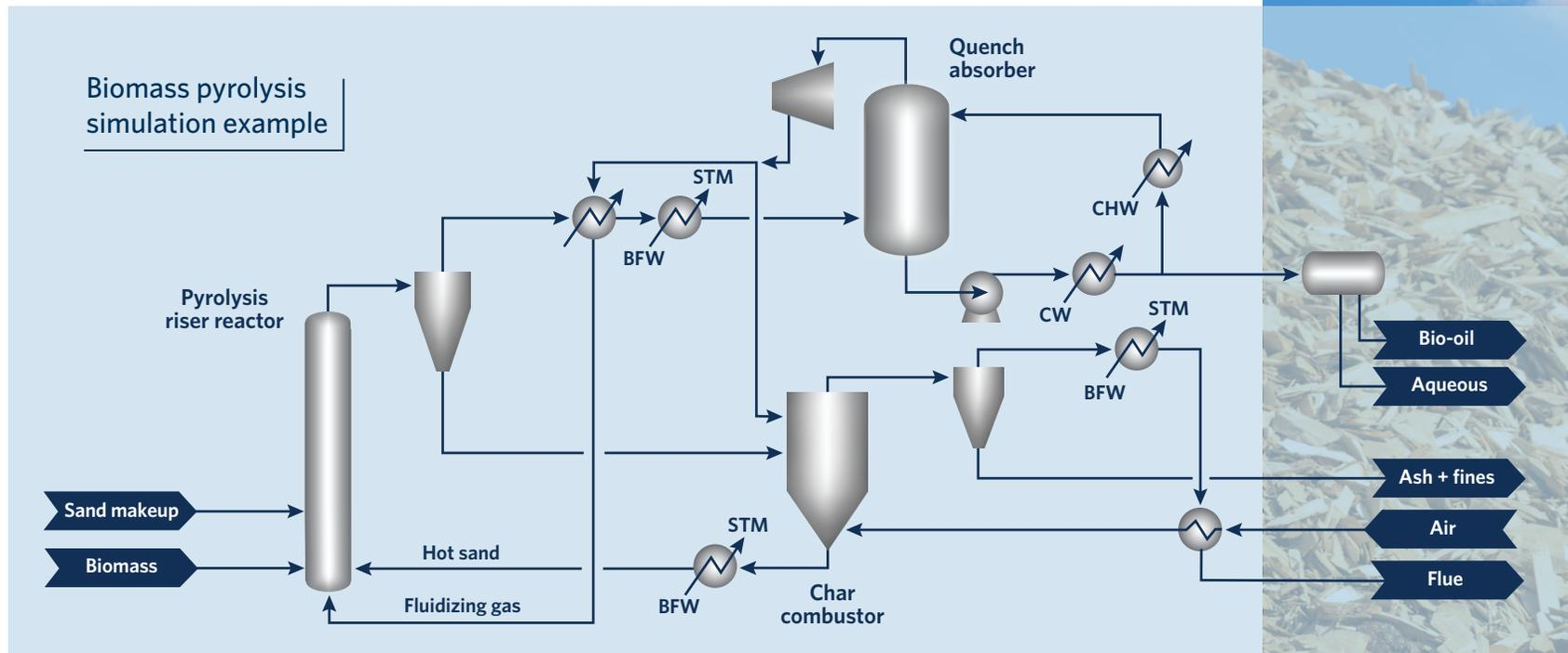
Figure 3. Biomass pyrolysis simulation example.
