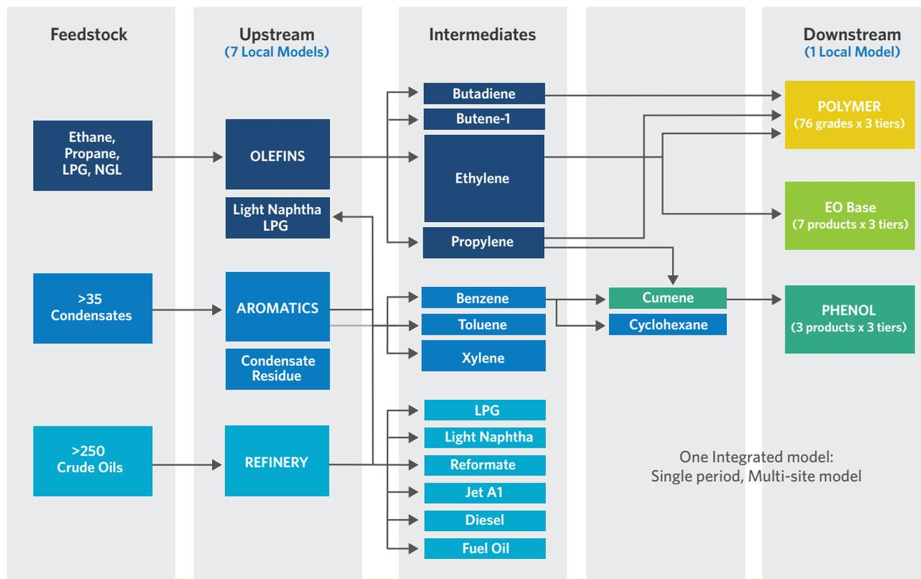
Figure 1. Aspen PIMS-AO enables short-term tactical planning and optimization for feedstock selection, production level and product mix, furnace line-ups, cracking severity/conversion optimization and energy usage.
