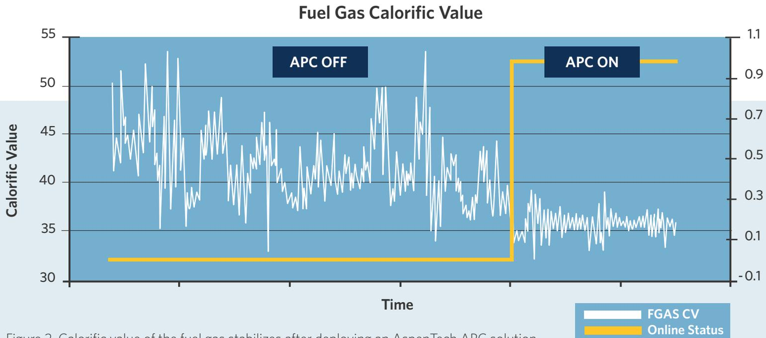
Figure 2. Calorific value of the fuel gas stabilizes after deploying an AspenTech APC solution.
