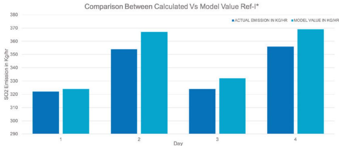
Figure E: SO<sub>2</sub> Emission from Ref-1 on 4 Various Sample Days
