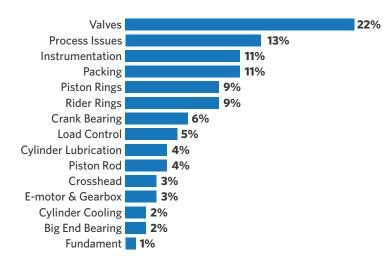
Figure 1: Most frequent failure modes of hyper compressors (source: *DIAGNOSTYKA, 2018, Vol. 19, No. 1*)
