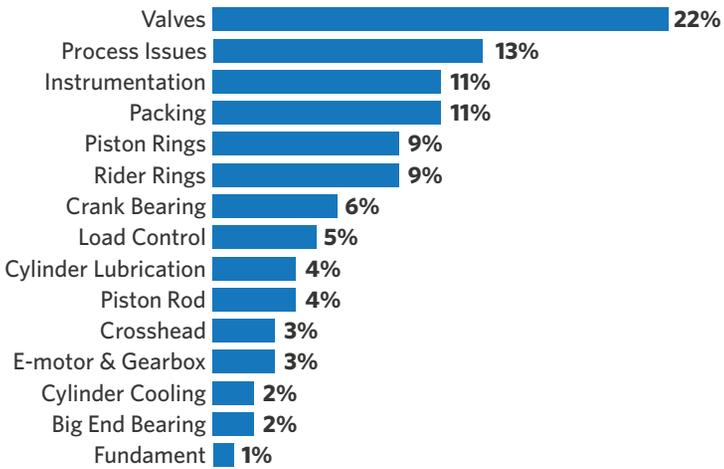
Figure 1: Most frequent failure modes of hyper compressors (source: *DIAGNOSTYKA, 2018, Vol. 19, No. 1*)
