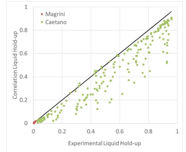
**Figure 8:** Comparison of the liquid hold-up between the calculated and experimental results in a vertical geometry
