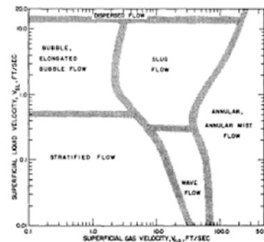
**Figure 1:** (a) Determining the pressure gradient for the flow of a multiphase fluid in a pipe. The flow regime map shown is from Mandhane, J.M., et al. (1997)
