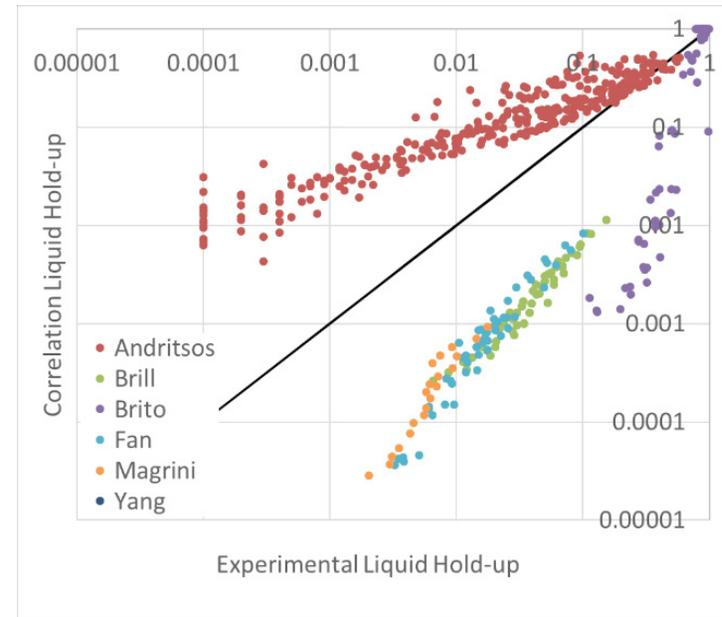
Figure 4: Comparison of the liquid hold-up between calculated and experimental results in a horizontal geometry
