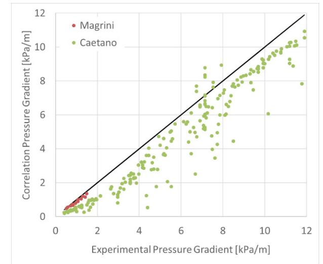
**Figure 7:** Comparison of the pressure gradient between the calculated and experimental results in a vertical geometry
