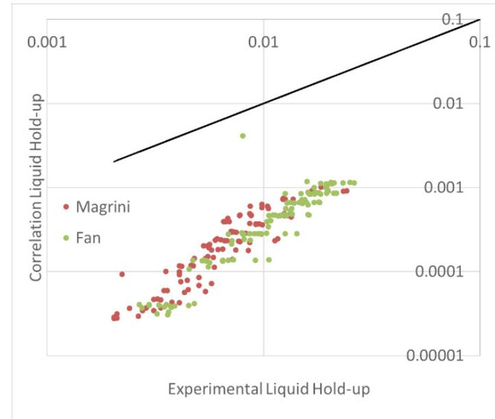
**Figure 6:** Comparison of the liquid hold-up between the calculated and experimental results in an inclined geometry
