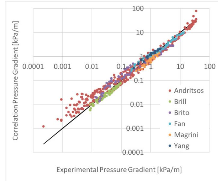
**Figure 3:** Comparison of the pressure gradient between calculated and experimental results in a horizontal geometry
