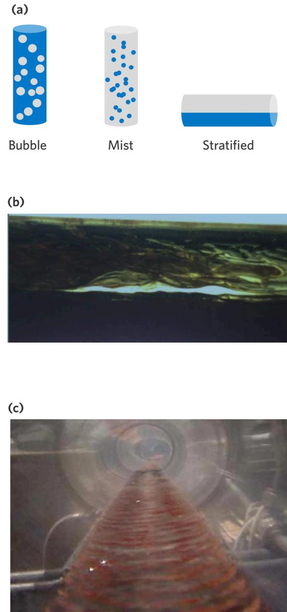
**Figure 1:** (a) Schematic examples of flow regimes in multiphase pipe flow. (b) Experimental flow regime formed during oil-gas flow1. (c) Stratified wavy flow pattern for oil-air flow2.
