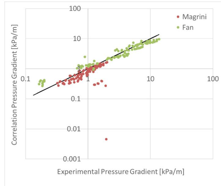
**Figure 5:** Comparison of the pressure gradient between the calculated and experimental results in an inclined geometry
