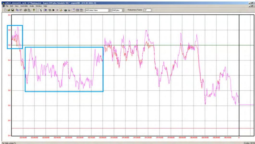
Figure 6: The CV LP steady-state target is underneath the actual CV value, while the MV target is held constant
