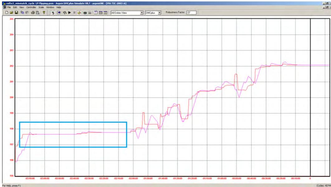
Figure 5: The MV target may be constant for long periods of time if the CV is still near the optimal solution and is not violating constraints
