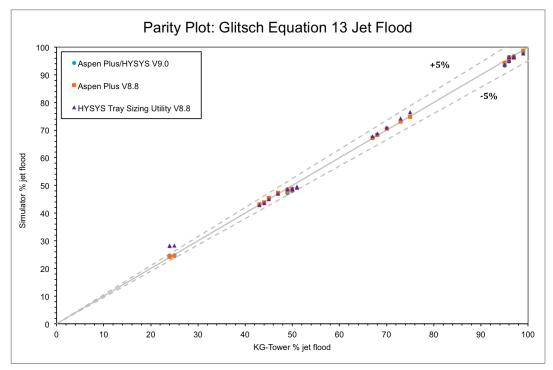
Figure 9: Parity plot comparing sieve tray approaches to jet flood calculated by previous versions of Aspen Plus and Aspen HYSYS and the new versions of Aspen Plus and Aspen HYSYS with those from KG-TOWER. Glistch Equation 13 was used for this comparison.
