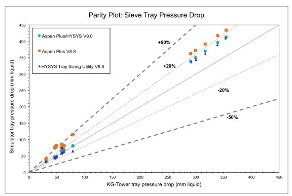
Figure 7: Parity plot comparing sieve tray pressure drops calculated by previous versions of Aspen Plus and Aspen HYSYS and the new versions of Aspen Plus and Aspen HYSYS with those from KG-TOWER.
