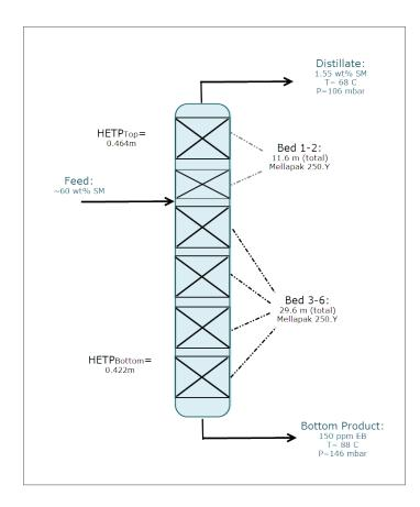
Figure 14: Diagram of the ethylbenzene/styrene splitter example
