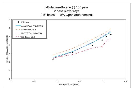
Figure 11: This chart compares the tray pressure drops calculated by the new Column Analysis feature in Aspen Plus and Aspen HYSYS with data from an FRI experiment.<sup>17</sup>
