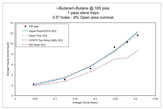
Figure 10: This chart compares the tray pressure drops calculated by the new Column Analysis feature in Aspen Plus and Aspen HYSYS with data from an FRI experiment.<sup>16</sup>
