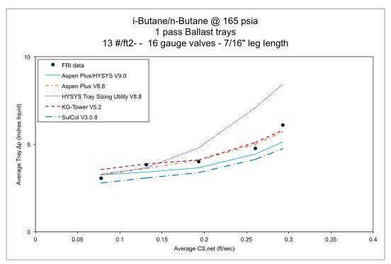
Figure 12: This chart compares the tray pressure drops calculated by the new Column Analysis feature in Aspen Plus and Aspen HYSYS with data from an FRI experiment.<sup>4</sup>
