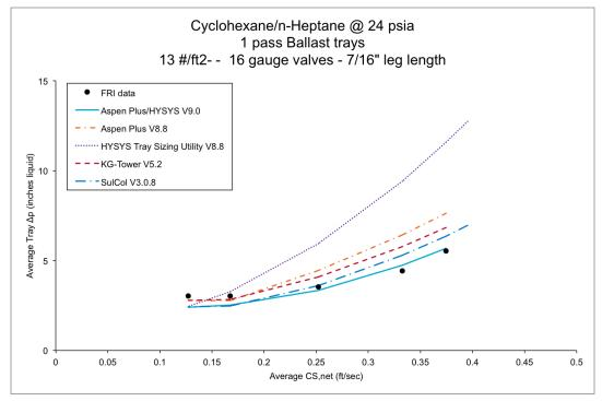
Figure 13: This chart compares the new Column Analysis feature in Aspen Plus and Aspen HYSYS with data from an FRI experiment.<sup>4</sup>
