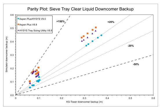
Figure 8: Parity plot comparing sieve tray downcomer backups calculated by previous versions of Aspen Plus and Aspen HYSYS and the new versions of Aspen Plus and Aspen HYSYS with those from KG-TOWER
