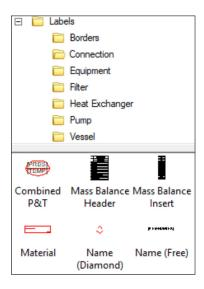
30. Go to Labels | Equipment to add smart labels for equipment. Use the Name (5mm) label. There are specific labels for Heat Exchangers and Pumps in the corresponding folders that can be added to the PFD. Labels will automatically display data from the transferred simulation data now stored in the ABE database.
