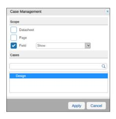
**15.** Click **Apply**. Return to the datasheet and confirm the DESIGN FLOW CASE column is filled. This datasheet lets users display the data from multiple case on the same page.
