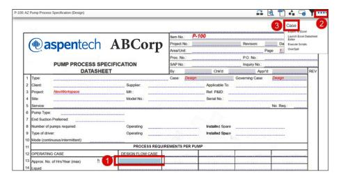
**14.** The **Case Management** window displays. Fill in the case information for the selected column in the datasheet. Check the **Field** option and confirm the option **Show** is selected on the dropdown list next to it. Finally, indicate the case to display (Design).
