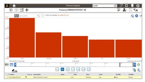
With aspenONE<sup>®</sup> Process Explorer<sup>™</sup>, users can display time-in-state analysis for a batch reactor. The height of each bar represents the amount of time the reactor was in a different state.
