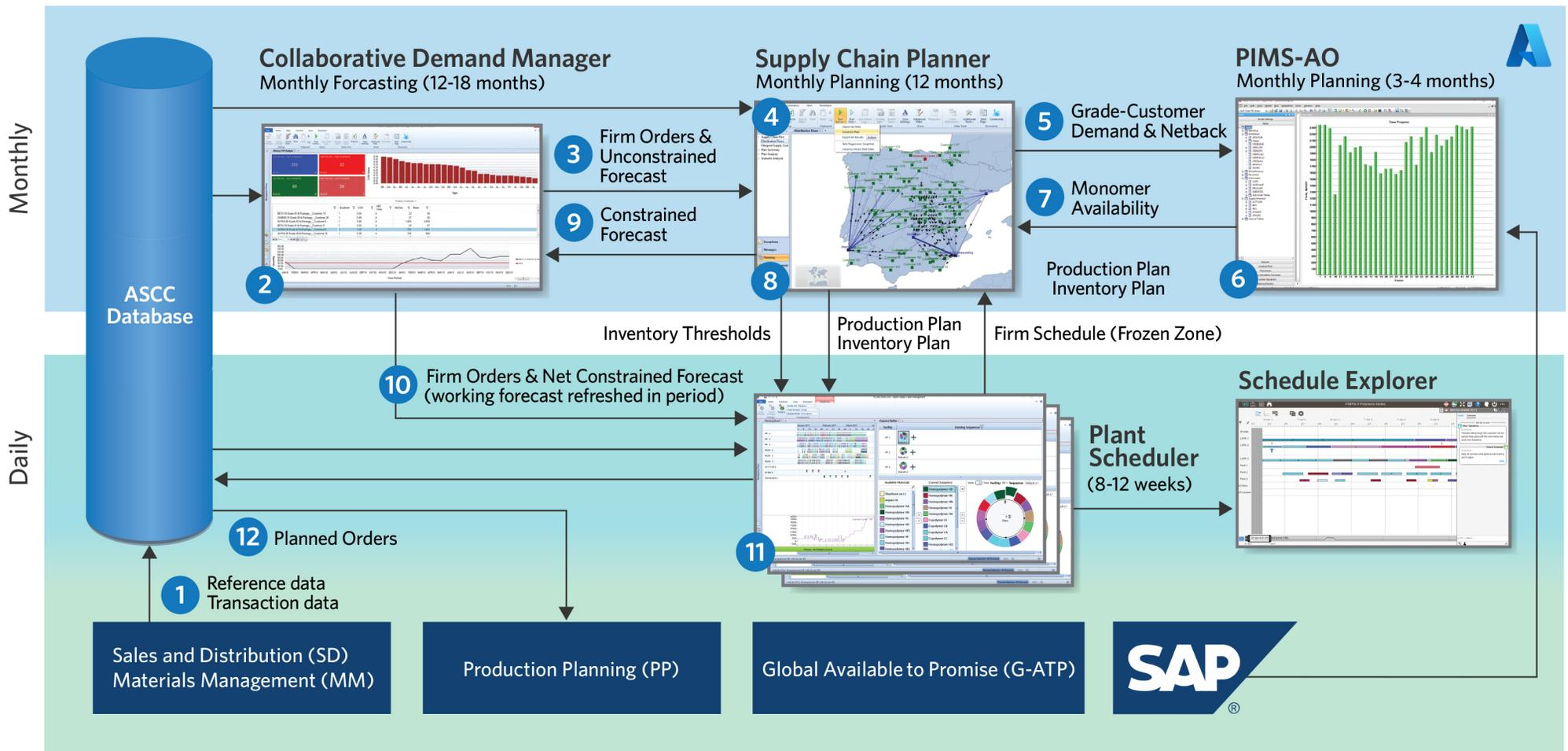
Figure 2. Business process diagram with step-by-step processes, data and decision flows. SCP, PS, CDM and ASE are running in Azure private cloud.
