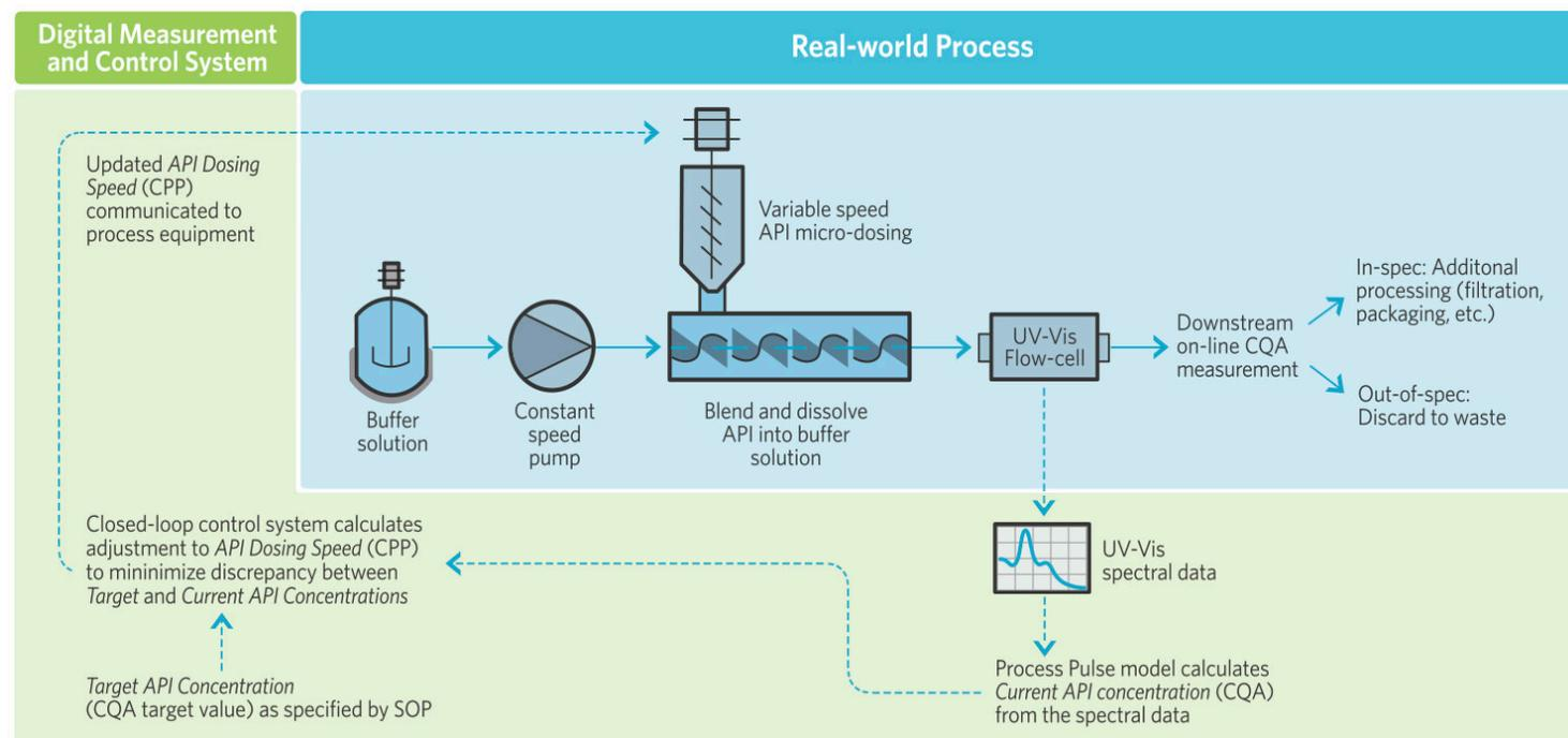
Figure 2. Closed-loop control system in production.
