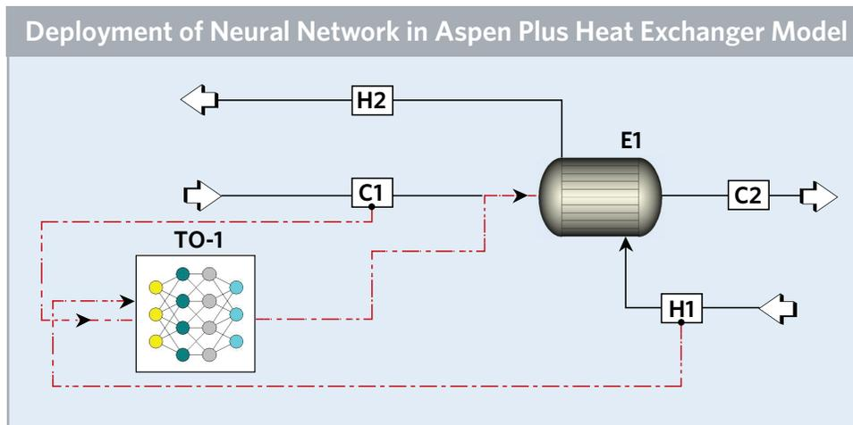
The neural network is deployed inside Aspen Plus to improve model predictions.
