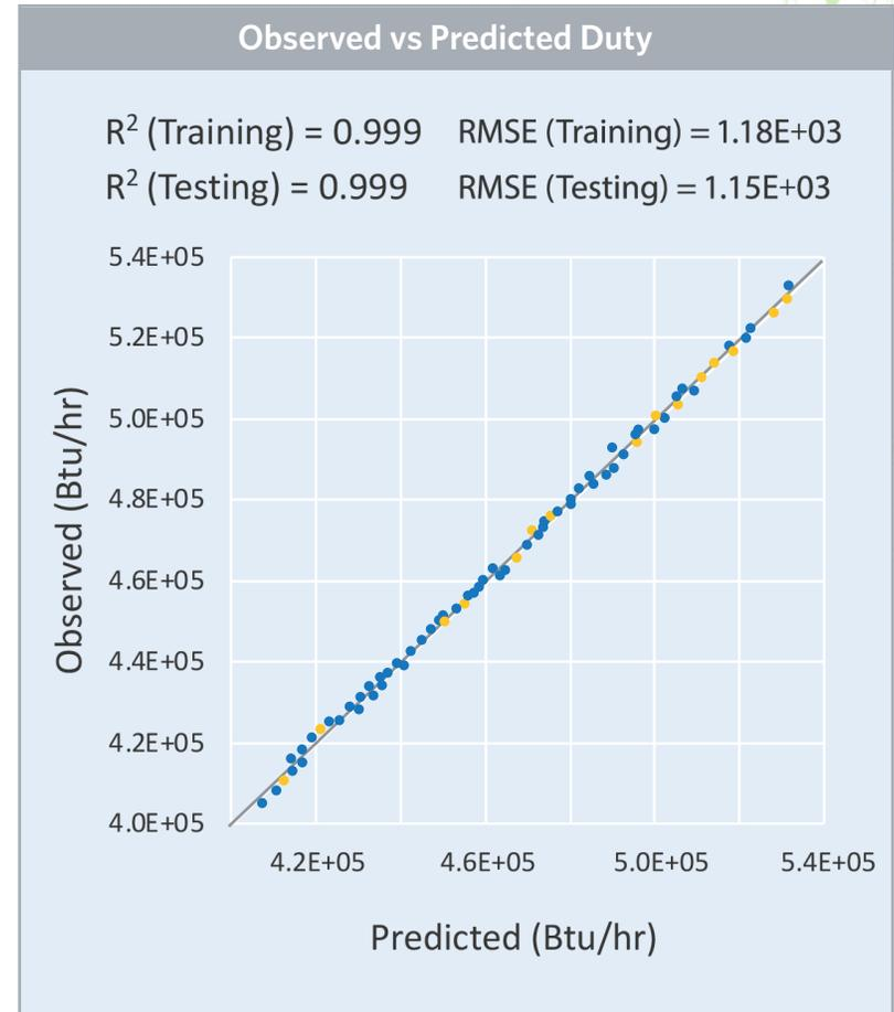
Duty calculations with hybrid models have a 99.9% accuracy rate compared to plant data.
