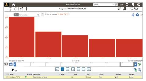
With aspenONE<sup>®</sup> Process Explorer<sup>™</sup>, users can display time-in-state analysis for a batch reactor. The height of each bar represents the amount of time the reactor was in a different state.
