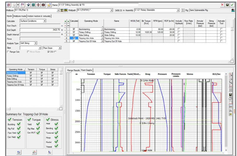
Torque & Drag dialog with inputs and results.
