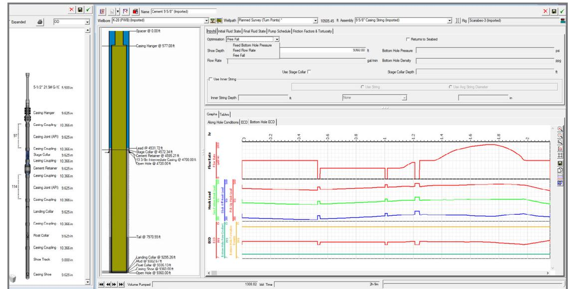
Casing string defined using Sysdrill Assembly Builder, cementing dialog with fluid schematic and associated ECC plot.
