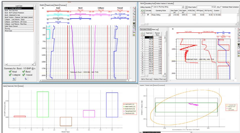
Casing and tubing analysis dialog with inputs and results, casing wear calculations and casing stretch bar graph.
