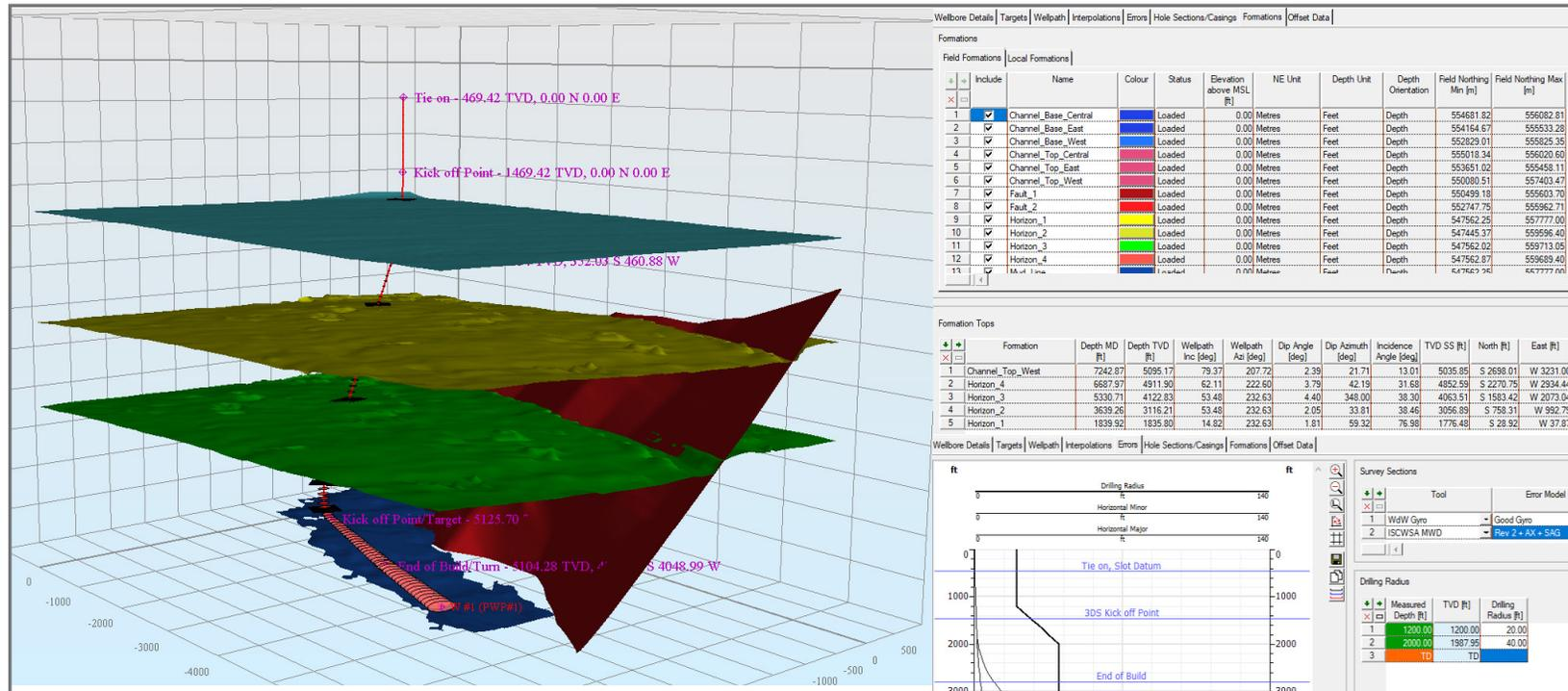
Wells and geological formations shown in Sysdrill 3D view. Well intersections and error model details.
