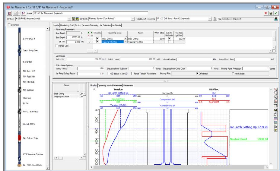
Jar placement module determines optimal location for Jars.
