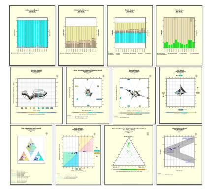
Figure 3. Water analysis graphic plots in Geolog help define the origin of the water, physical properties and tendency to precipitate.
