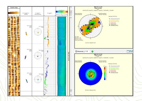
Figure 1. Image log interpretation for dip and fracture interpretation in Aspen Geolog.
