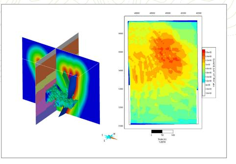
Figure 2. 3D play fairway analysis (left) and heat-in-place per m<sup>2</sup> map (right) of a geothermal field in SKUA-GOCAD.
