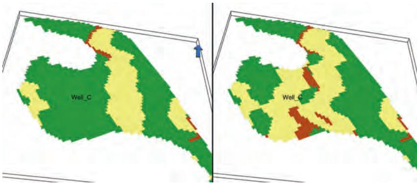
**Figure 4** Illustration of a locally updated channel model. Left shows the original facies model where channel objects have been modelled, prior to Well\_C being drilled. Right shows the locally updated facies model where the newly drilled Well\_C is conditioned to.
