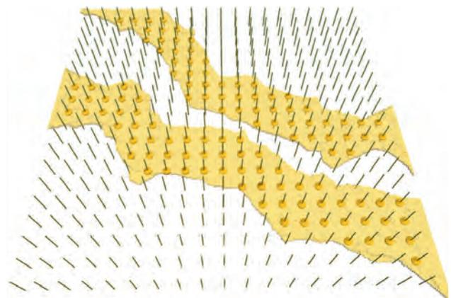
**Figure 6** A synthetic case with more than 300 densely spaced wells demonstrating the effectiveness of the new algorithm in conditioning on many observations of an object, while avoiding areas with background observations (after Hauge et al., 2017).
