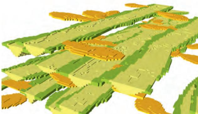
**Figure 5** The new Next Generation Object Modelling Algorithm can model meandering channels and channel belts.
