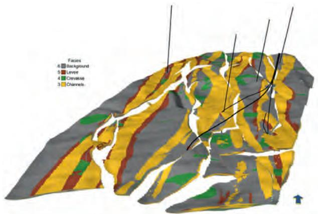
**Figure 8** Channel, levees and crevasses are all linked together with an erosional hierarchy, which leads to geologically realistic facies deposits consistent with well data.
