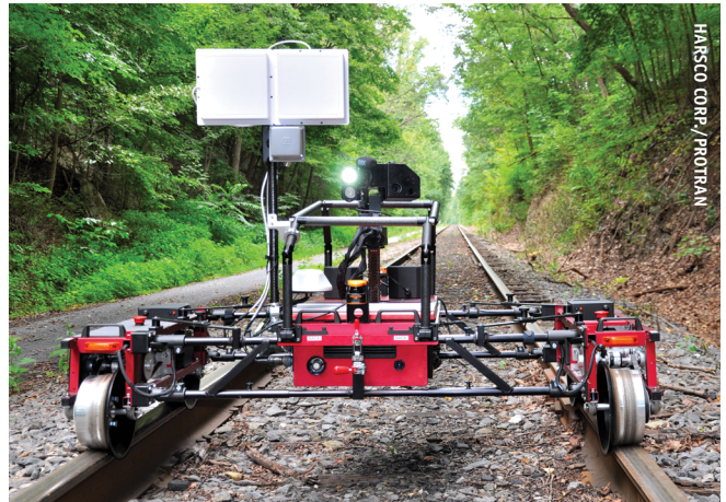
The new Instrumented Rail inspection System, or IRIS, is a robotic vehicle that can be operated remotely from a portable base station for security inspection and emergency first response work.
