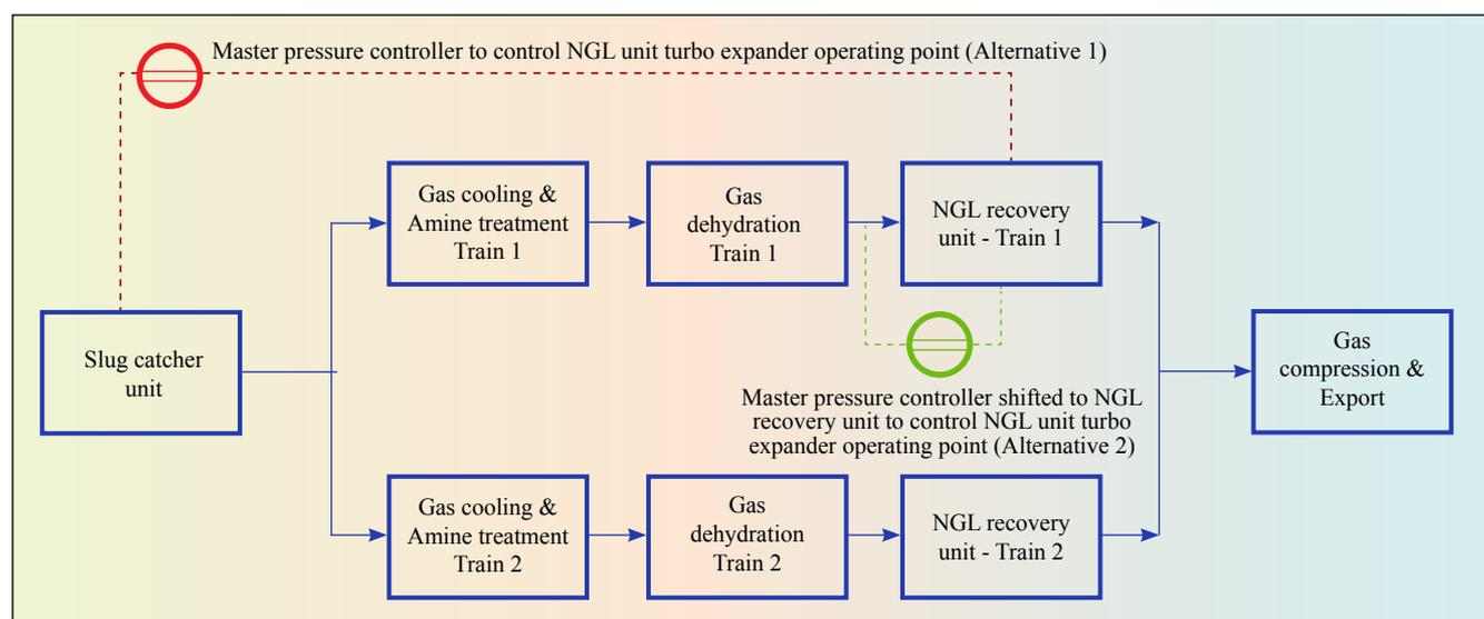
Figure 4: Block flow diagram of NGL recovery unit in the overall gas plant
