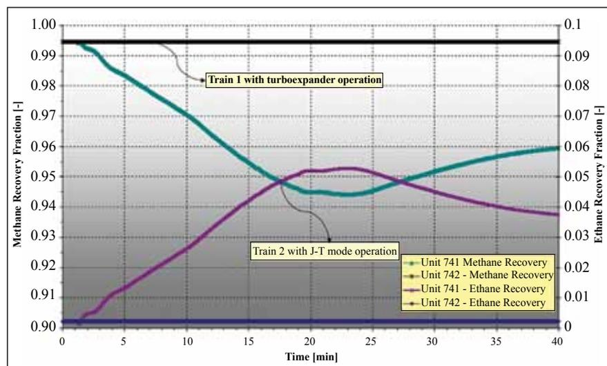
Figure 6: Stable column recoveries by localizing the master pressure control
