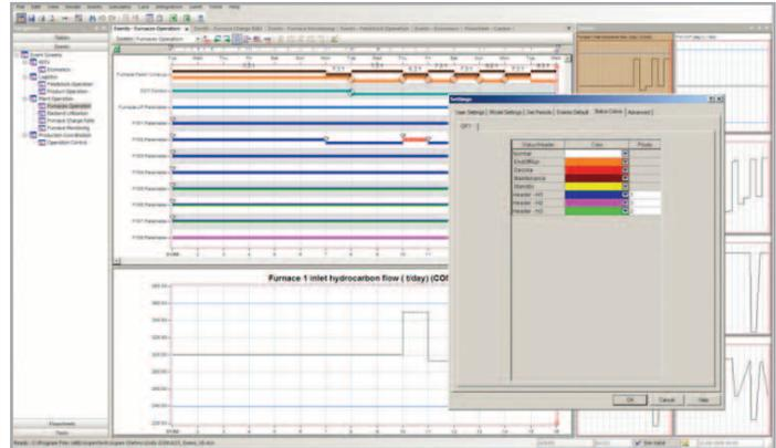
*Aspen Olefins Scheduler* uses feed headers to enable the scheduling of complex furnace line-ups
